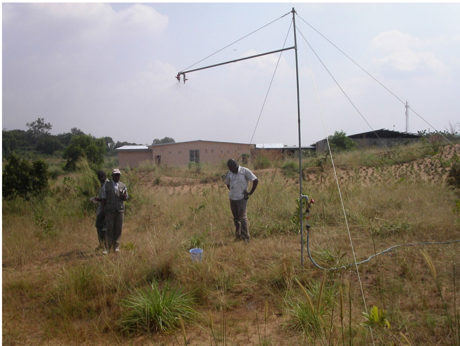
Fig. 5 KU Leuven rain simulator deployed in the ERAIFT site. The wetted impluvium is visible in the foreground
